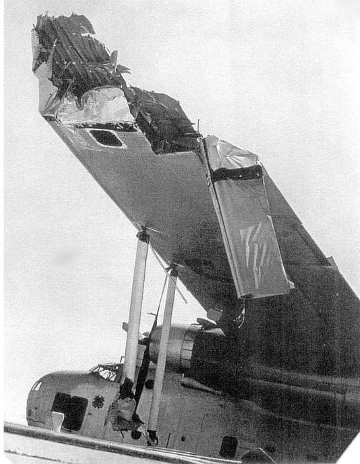
Showing the damage to the left wingtip and aileron, and the struts to the missing left wingfloat.
