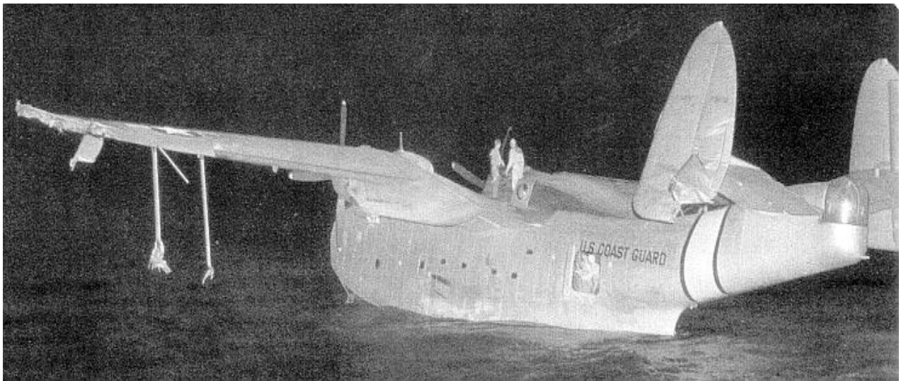
U.S. Coast Guard PBM-5 59012 at rest on the small sand spit (Sport Island) adjacent to Dinner Key CGAS, Miami, Florida, April 8, 1948. This photo is not a negative - it was taken using a high-powered flash! Note the damaged left wing tip and aileron, and missing left wing float.
