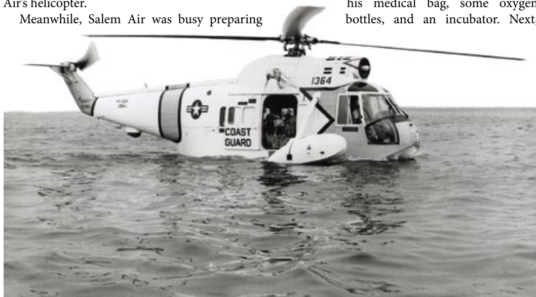
Facing page, top: The Soviet factory ship, Trudovaja Slava. Author's collection Above: The HH-52A Sea Guardian, built by Sikorsky Aircraft Company, was powered by a 1,250shp General Electric T58-GE-8 turboshaft engine. The HH-52A was fully amphibious and had several features for the search-and-rescue role, including a folding platform along the side of the fuselage and a hoist above the door. It had a maximum speed of 110 miles per hour and a capacity of more than 3,000 pounds. USN Photo/EBNAL
