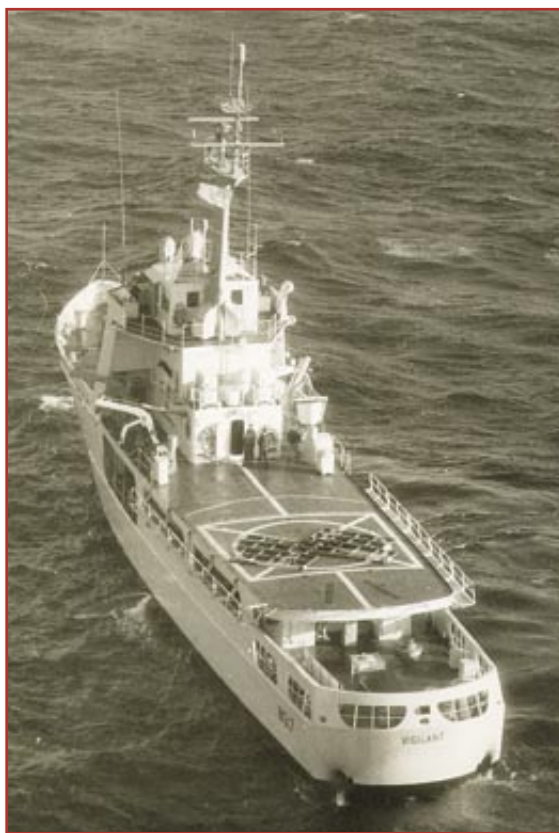
Vigilant is a Reliance-class medium endurance cutter 210-feet in length, with a beam of 34 feet and a displacement of 1,000 tons. Her two diesel engines produce a top speed of 18 knots. She has a crew of 75 and was commissioned in October 1964 in Cape Canaveral, Florida. Author's collection
