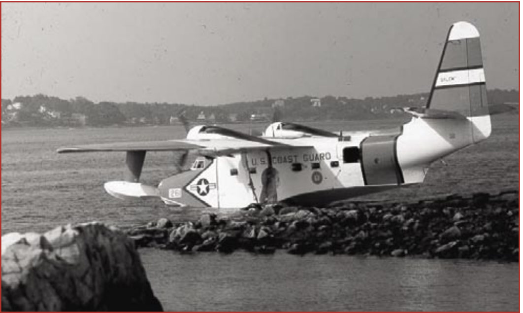
A Grumman HU-16 Albatross taxis over the side at Salem Air Station. The Albatross featured a conventional two-step hull into the sides of which the main wheels retracted and a high wing with fixed stabilizing floats. Author's collection
