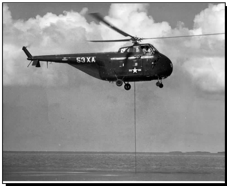
HO4S with Pratt-Whitney 1340 engine and AN/ASQ-4 sonar - 1952
