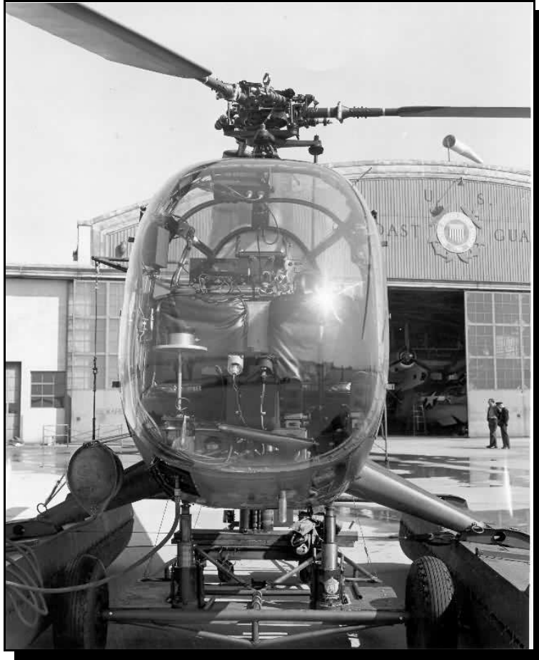
XHOS Helo with Hayes sonar installed
