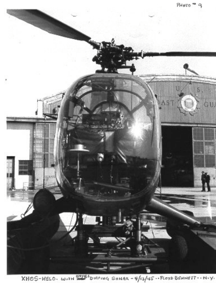
XHOS-HELICOPTER WITH DIPPING SONAR - 4/13/45 - FLOYD BENNETT - N.Y.
