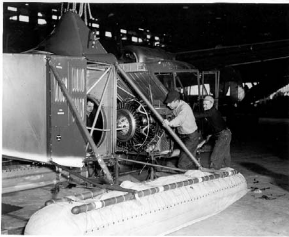
The Coast Guard crew reassembles the HNS in the hangar. Chief Forest Giles, AM1 Irv Eifferblatt and AM1 Gus Jablonski maneuver the front assembly into position to mate with the gearbox and tail assemblies.
