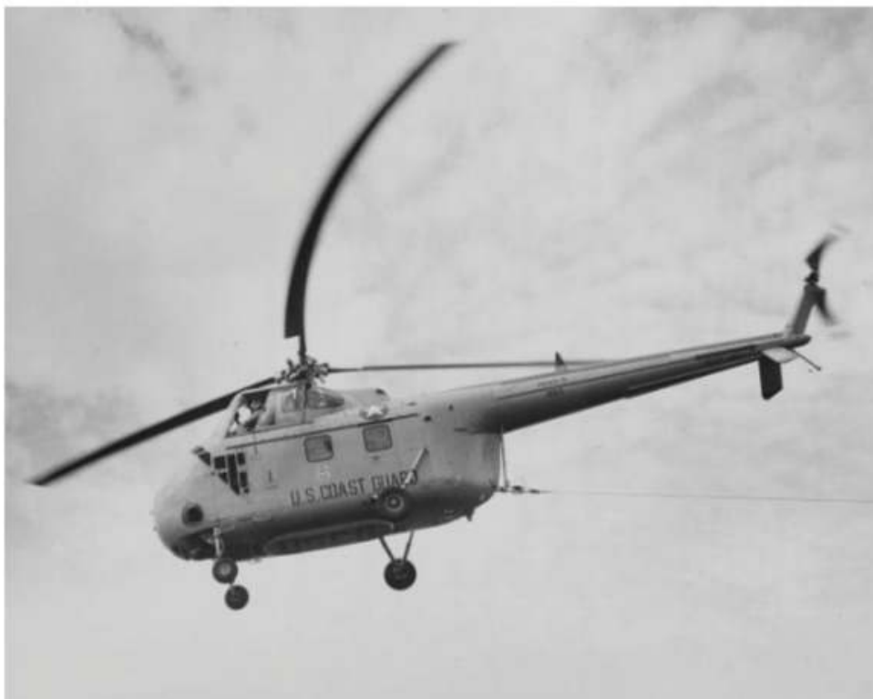
A closeup shows the steel cable attached to a U.S. Coast Guard HO4S-3G helicopter used to tow the 75-ton buoy tender Birch during tests recently conducted under "Project Tugbird" at the U.S. Coast Guard Air Station at St. Petersburg, Florida in 1958. (U.S. Naval Institute Photo Archive)
