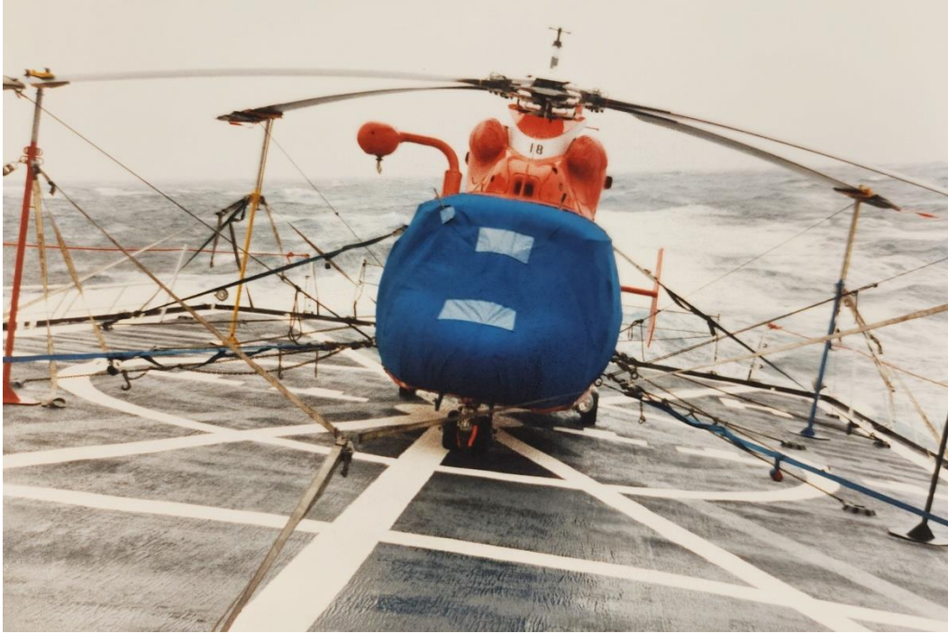
PHOTO CAPTION (Rick Stanchi): ALPAT mechanic AM2 Chris Wagner is credited with conceptualizing and manufacturing blade restraining devices. This new equipment precluded pulling the blades in winds up to about 90 knots.
